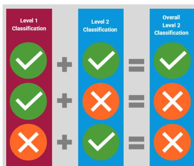
Figure 4: Example of Level 2 data integration with Level 1 using a one out, all out approach
