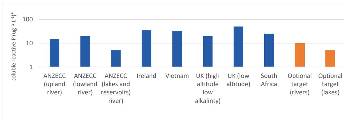
Figure 8: Examples of soluble reactive phosphate concentration targets used in countries (Source: data from multiple sources, refer to Annex 1)
